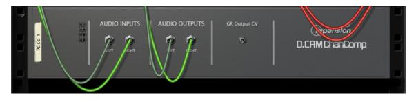
DCAM ChanComp features a set of various inputs and outputs on its rear panel.
