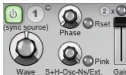
Cypher's Ext. external audio input appears in place of the white Noise source in each osc. The Pink button must be deactivated.
