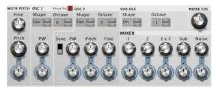
The oscillators feature an audio-rate Min/Max function which is introduced via the **1x2** fader in the Mixer section. This function creates complex timbres reminiscent of FM, cross-modulation or ring-modulation.
