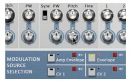
Note that the LED above the Osc 2 **Pitch** TransMod amount knob has turned *yellow* - this indicates that the knob features a modulation depth for the *current source*.
